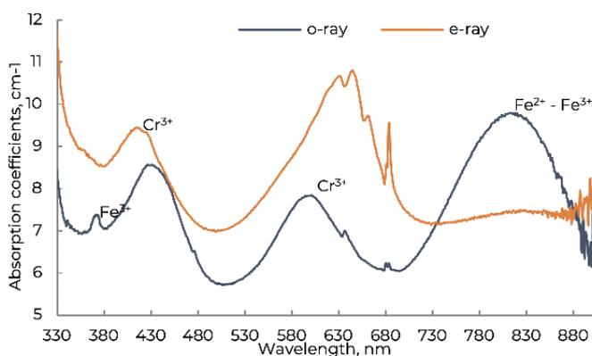
Figure 15: UV-Vis-NIR spectra (o and e rays) of an emerald from the Elmeki region in Niger (0.17 carat stone in figure 6 which contains about 1000 ppm of chromium, 300 of vanadium and 4000 of iron). The main chromophoric elements are chromium and iron.
