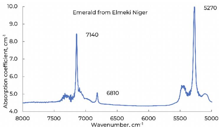
Figure 16: FTIR Spectrum of the same 0.17ct Niger emerald as used for the UV-vis-NIR, Figure 15. Peaks due to the presence of water in the emerald channels.
